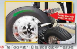
runout (eccentricity) of a tire and wheel assembly.
